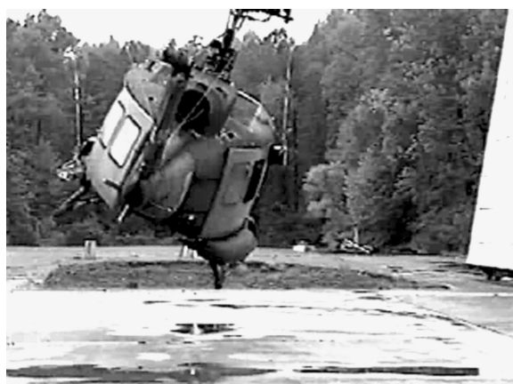
Fig. 18 Pretest UH-1 Huey helicopter with external fuel tank.
