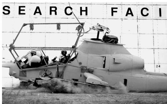
Fig. 17 Crash test of the AH-1S helicopter with crew restraint systems.
