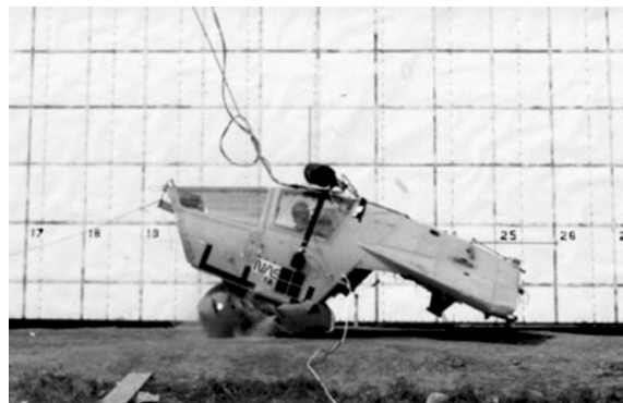
Fig. 19 F-111 crew escape module with airbag attenuation system.
